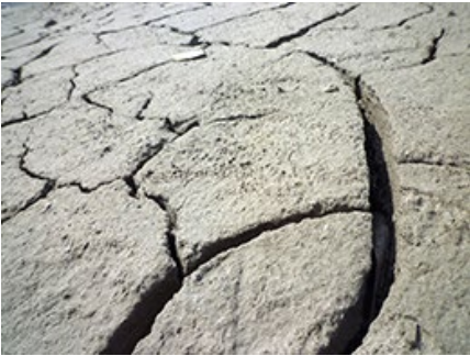
An example of how clay soil reacts in a drought.
