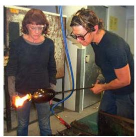
"While blowing glass at a temperature of about 1150C, organic material was inserted into one end of the egg-shaped spheres - like a ship in a bottle. When the eggs were closed, the pine cones and other organic objects began to burn. Although reduced to carbon, they still held their form inside the spheres," Bisetto said.
