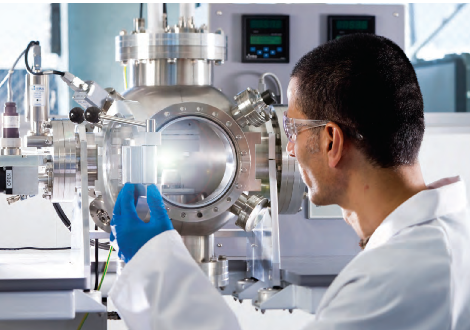
A researcher using the Mawson Institute's microplasma reactor, which is used for research on the surface engineering of microplasma at the Mawson and Ian Wark Research institutes. This research is showing exciting potential for medical and industrial applications.
