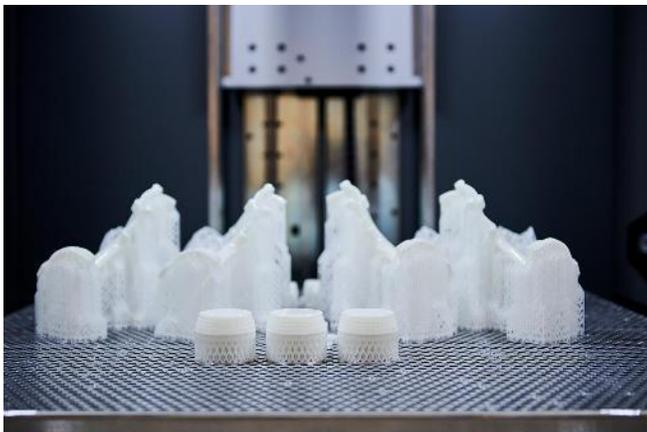
Build complex parts with smooth finishes due to exceptional layer to layer scan repeatability. SLA offers users the ability to produce parts for a range of different applications, requiring different properties, with one technology
